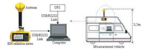
Figure 2. Equipment and vehicle used for the measurements.
