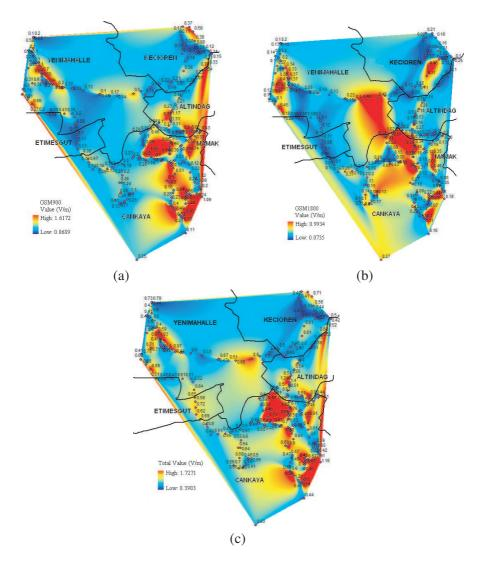
**Figure 5.** Electric field values E (V/m) measured (a) for GSM900 base stations, (b) for GSM1800 base stations, (c) total E (V/m) values.
