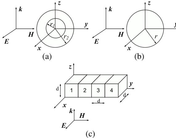
**Figure 3.** Geometries of bi-anisotropic objects considered as numerical examples. (a) A gyroelectric spherical shell, inner radius  $r_1 = 0.3\lambda_0$ , outer radius  $r_2 = 0.6\lambda_0$ . (b) A chiral sphere, radius  $r = 0.8\lambda_0$ . (c) A bi-anisotropic cubes,  $d = \lambda_0$ .
