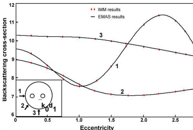
**Figure 9.** Backscattering cross-section of a dielectric cylinder with two inclusions as functions of eccentricity.
