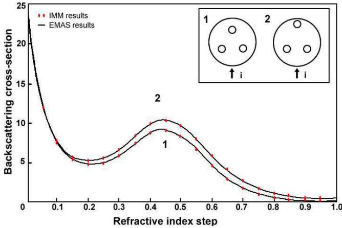
**Figure 7.** Backscattering cross-section of a dielectric cylinder with three inclusions as functions of refractive index step.
