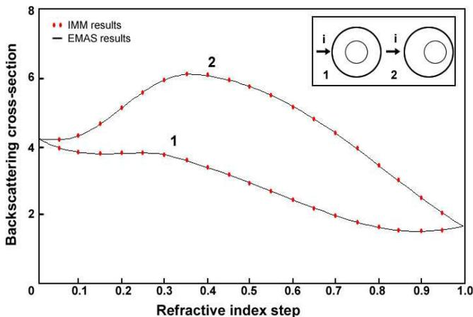
**Figure 5.** Backscattering cross-section of a dielectric cylinder with one inclusion as functions of refractive index step.
