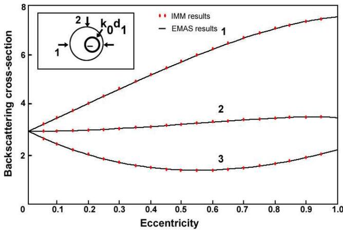
**Figure 8.** Backscattering cross-section of a dielectric cylinder with one inclusion as functions of eccentricity.
