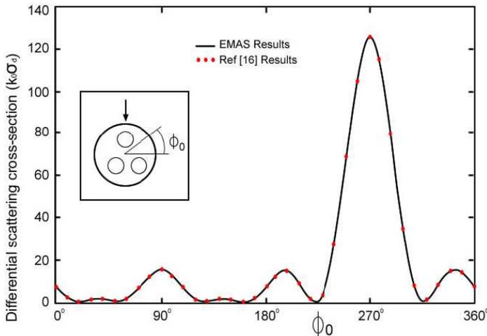
**Figure 4.** Differential scattering cross-section of cylinder with three inclusions of air holes as functions of observation angle.
