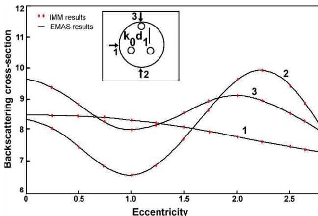
**Figure 10.** Backscattering cross-section of a dielectric cylinder with three inclusions as functions of eccentricity.
