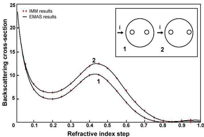
**Figure 6.** Backscattering cross-section of a dielectric cylinder with two inclusions as functions of refractive index step.
