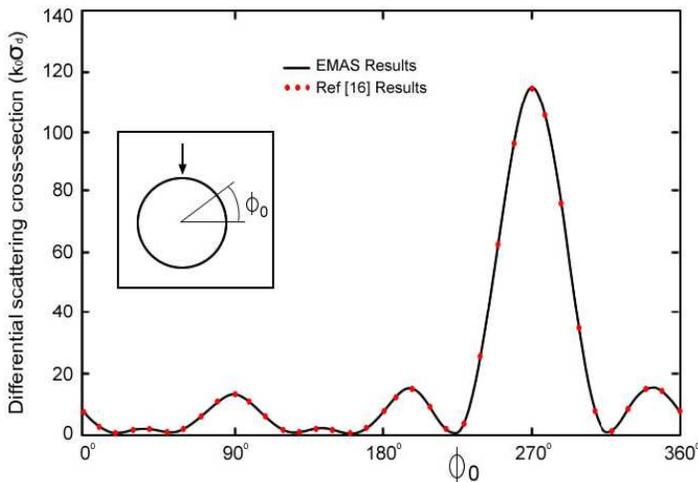
**Figure 3.** Differential scattering cross-section of a dielectric cylinder as functions of observation angle.
