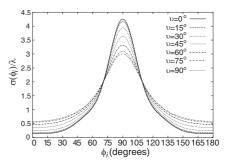
Figure 3. Variation of the normalized backscattering width with the angle of incidence, for elliptic cylinders of axial ratio 2,  $ka = \pi$ , and different v.
