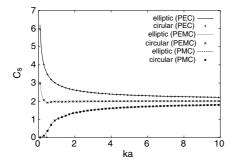
Figure 2.  $C_s$  versus ka for an elliptic cylinder of axial ratio  $\approx 1$  and for a circular cylinder, when  $MZ = 0, 1, \infty$ .
