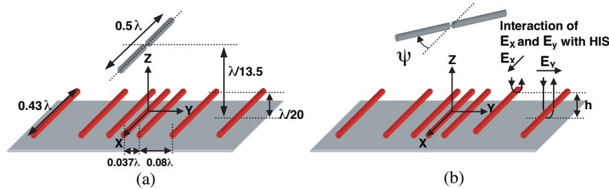
**Figure 1.** (a) The dipole antenna over the NU-HIS in [5], (b) applying rotation to obtain circular polarization.
