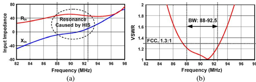
**Figure 3.** Impedance matching characteristics for the structure in Figure 2, (a) input impedance, (b) VSWR.
