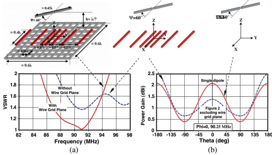
**Figure 5.** (a) VSWR of the structure in Figure 2 with and without the wire grid plane, (b) radiation pattern for the structure in Figure 2 without the wire grid plane together with that for a single dipole in free space.
