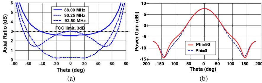
**Figure 4.** Axial ratio and radiation pattern for the structure in Figure 2, (a) axial ratio in  $\Phi = 90^\circ$  plane, at both edges of the desired frequency range, (b) radiation pattern at 90.25 MHz.
