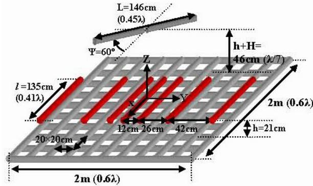
**Figure 2.** The dipole antenna over the NU-HIS in [5], optimized to be a standard circularly polarized FM broadcasting antenna; the radius for all wires is 1.6 cm ( $\approx \lambda/200$ ).
