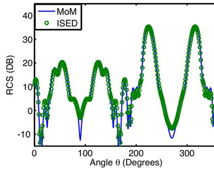
**Figure 18.** Radar cross-sections of the triangular periodic structure shown in Fig. 16 under the oblique incidence of plane waves ( $\theta_i = 45^\circ$ ).
