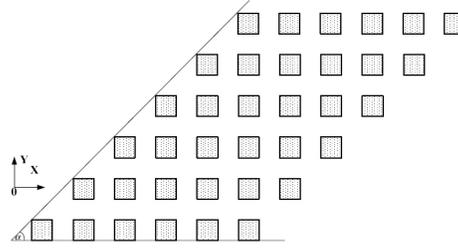
**Figure 10.** Parallelogrammic periodic structure where the square PEC patch element has a size of  $\lambda \times \lambda$ , the gap between two cells is equal  $1\lambda$ , and  $\alpha = 45^\circ$ ,  $N_x = 6, N_y = 6, N_C = N_x \times N_y = 36$ .
