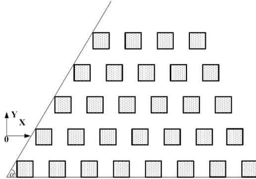
**Figure 13.** Trapeziform periodic structure where the square PEC patch element has a size of  $\lambda \times \lambda$ , the gap between two cells is equal  $1\lambda$ , and  $\alpha = 60^\circ$ ,  $N_{xl} = 8$ ,  $N_{xu} = 4$ ,  $N_y = 5$ ,  $N_C = (N_{xl} + N_{xu})N_y/2 = 30$ .
