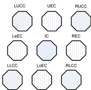
**Figure 7.** Small problem containing all kinds of ISED basis functions in the parallelogrammic periodic structure.
