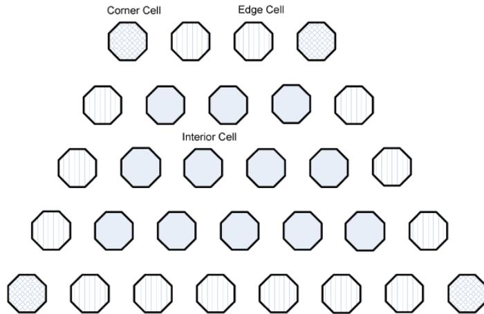
**Figure 2.** Supports of different types of ISED basis functions in the trapeziform periodic structure.
