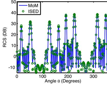
**Figure 12.** Radar cross-sections of the parallelogrammic periodic structure shown in Fig. 10 under the oblique incidence of plane waves ( $\theta_i = 45^\circ$ ).
