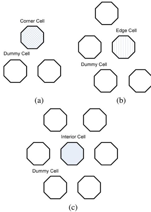
**Figure 6.** Dummy cells for different types of ISED basis functions in the triangular periodic structure.
