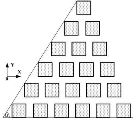
**Figure 16.** Triangular periodic structure where the square PEC patch element has a size of  $\lambda \times \lambda$ , the gap between two cells is equal  $1\lambda$ , and  $\alpha = 60^\circ$ ,  $N_x = 6$ ,  $N_y = 6$ ,  $N_C = (N_x + 1)N_y/2 = 21$ .
