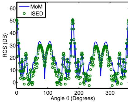
**Figure 14.** Radar cross-sections of the trapeziform periodic structure shown in Fig. 13 under the normal incidence of plane waves.
