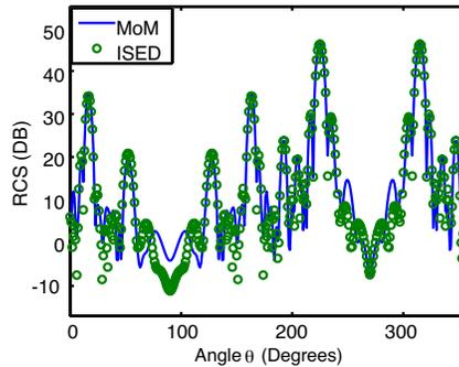
**Figure 15.** Radar cross-sections of the trapeziform periodic structure shown in Fig. 13 under the oblique incidence of plane waves ( $\theta_i = 45^\circ$ ).
