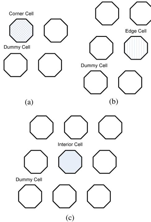
**Figure 4.** Dummy cells for different types of ISED basis functions in the parallelogrammic periodic structure.
