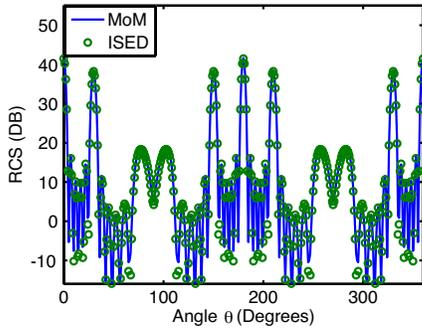
**Figure 11.** Radar cross-sections of the parallelogrammic periodic structure shown in Fig. 10 under the normal incidence of plane waves.
