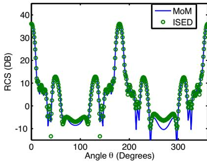
**Figure 17.** Radar cross-sections of the triangular periodic structure shown in Fig. 16 under the normal incidence of plane waves.
