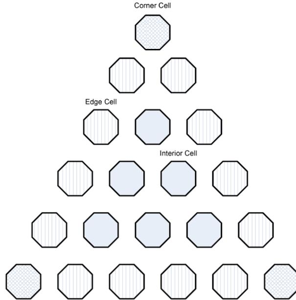
**Figure 3.** Supports of different types of ISED basis functions in the triangular periodic structure.
