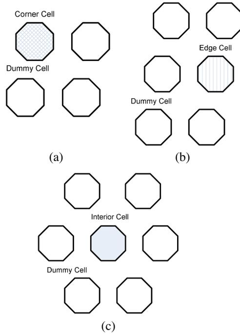
**Figure 5.** Dummy cells for different types of ISED basis functions in the trapeziform periodic structure.
