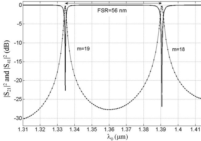
**Figure 5.** Scattering parameters of  $|S_{21}|^2$  (solid line) and  $|S_{41}|^2$  (dotted line) for two successive resonance modes of 18th and 19th for a microring resonator with  $W = g = 0.2 \mu\text{m}$ ,  $r_i = 1.6 \mu\text{m}$  and  $r_o = 1.8 \mu\text{m}$ .
