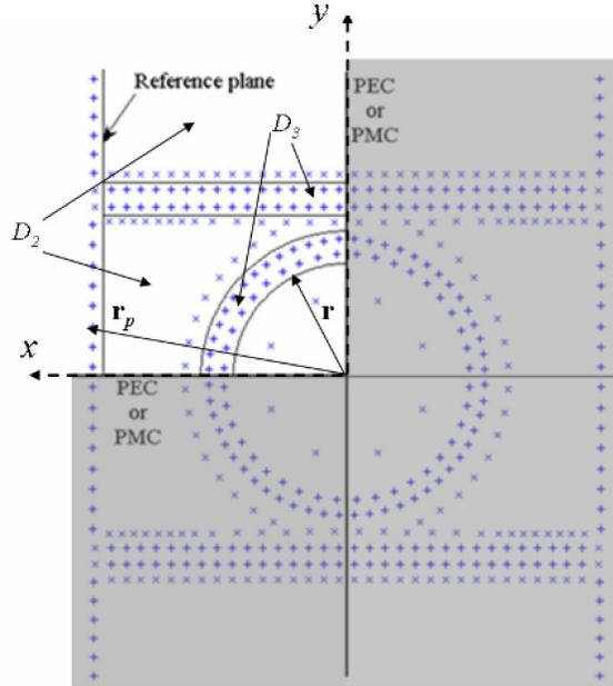
**Figure 3.** Location of the clusters of multipoles for expanding the fields of domain  $D_2$  is indicated by +, and for the fields of domain  $D_3$  is shown with  $\times$ , the mirror multipoles are located in the shaded region, and their amplitudes are given by the described rules.
