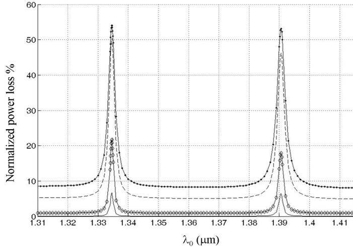
**Figure 8.** Normalized power loss (Equation (7)) for  $\tan(\delta) = 0$  (solid line),  $\tan(\delta) = 0.0001$  (diamond-line),  $\tan(\delta) = 0.0006$  (dashed line), and  $\tan(\delta) = 0.001$  (dotted line).
