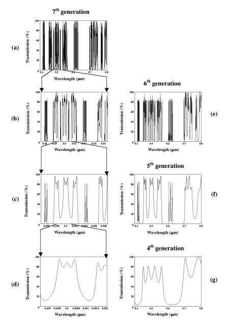
Figure 9. Autosimilarity aspect of transmission spectra of the generalized Fibonacci sequence FS (4, 1). Scalability can be seen clearly if one compares (a) with (e), and (c) with (f) and (d) with (g).
