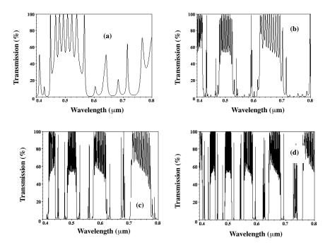
Figure 2. Transmission properties of a quarter-wave stack of the FS (1,m) system for the  $6^{th}$  generation at normal incidence as a function of wavelength for (a) m = 4; (b) m = 6; (c) m = 12; (d) m = 16.
