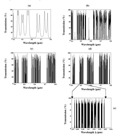
**Figure 7.** Transmission properties of a quarter-wave stack of the FS (n, 1) system for the  $6^{th}$  generation at normal incidence as a function of wavelength for (a) n = 2; (b) n = 6; (c) n = 10; (d) n = 12; (e) case n = 12 for the spectral range around the reference wavelength  $\lambda_0$ .
