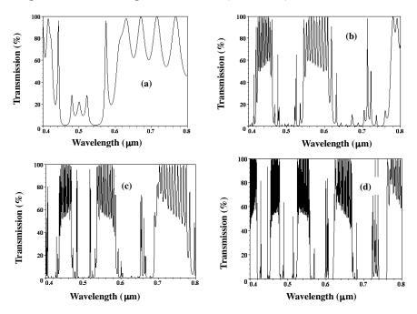
**Figure 5.** Transmission properties of a quarter-wave stack of the FS (1, m) system for the  $6^{th}$  generation at normal incidence as a function of wavelength for (a) m = 3; (b) m = 7; (c) m = 9; (d) m = 13.
