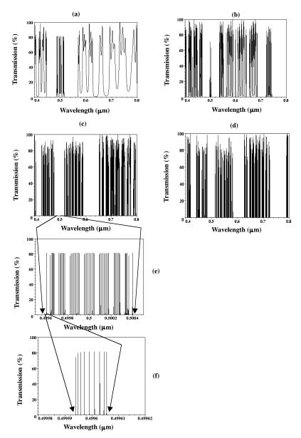
**Figure 8.** Transmission properties of a quarter-wave stack of the FS (n, 1) system for the  $6^{th}$  generation at normal incidence as a function of wavelength for (a) n = 3; (b) n = 5; (c) n = 9; (d) n = 11; (e) case n = 9 for the spectral range around the reference wavelength  $\lambda_0$ ; (f) case n = 9 for the spectral range around the wavelength 0.4996  $\mu$ m.
