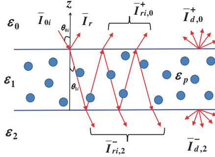
**Figure 1.** Diagram of the reflected intensity,  $\bar{I}_r$ , reduced intensity,  $\bar{I}_{ri}$ , and diffuse intensity,  $\bar{I}_d$  observed from a slab containing scatterers illuminated by an obliquely incident intensity,  $\bar{I}_{0i}$ .
