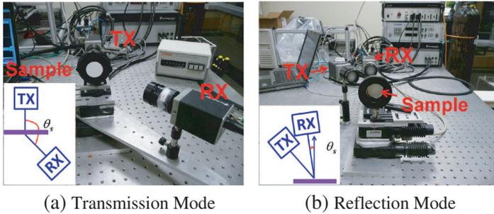
**Figure 2.** Experimental setup for (a) transmission measurement at a normal incidence,  $\theta_i = 0^\circ$  and  $\theta_s = 140^\circ$  and (b) reflection measurement at an oblique incidence,  $\theta_i = 29^\circ$  and  $\theta_s = -6^\circ$ .
